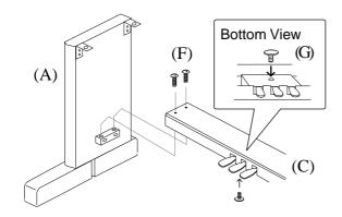
1. Insert the Adjuster (G) on the bottom of Pedal Board (C). Fasten (A) and (C) with four bolts (F).
